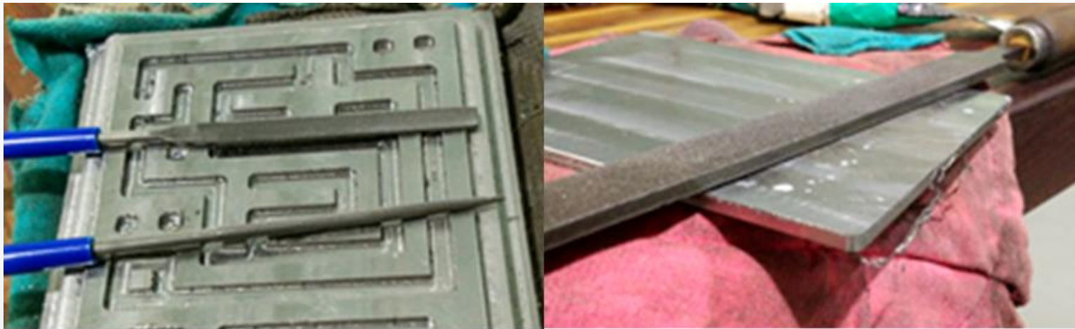
Figure 4: Deburring using needle and standard files
